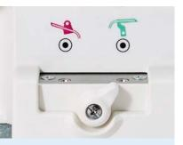
Looper selection lever Simply position your thread and direct the looper selection lever to the looper you wish to thread; to the right for 'threading' the lower looper and to the left for threading the upper looper.
