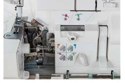
Adjustable foot pressure dial Simply dial 'N' for normal sewing. There are five-levels of presser foot adjustment to help feed heavy and lightweight fabrics.
